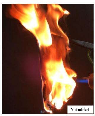
XTest with soft PVC sheet. Plasticizer 75 phr. Sample thickness: 2.5 mm.
